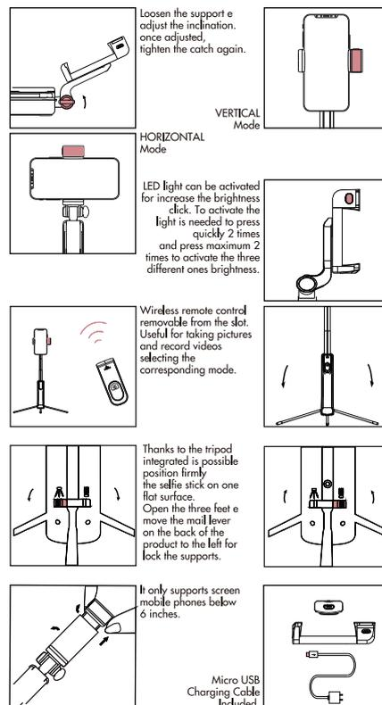
Loosen the support e adjust the inclination. once adjusted, tighten the catch again.
